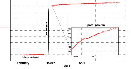
This plot from a GPS receiver in northern Japan tracks the station's daily positional changes along an east-west axis in the month before and the two and a half months after the March 11 earthquake. Having this kind of data covering all the phases of the seismic cycle is critical for developing detailed mechanical models of fault systems.
