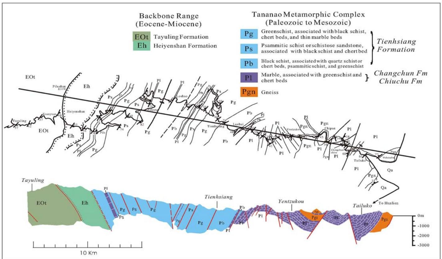
Fig. 2. Geologic road map of the eastern part of the Central Cross-Island Highway (After Chen, 1979)
