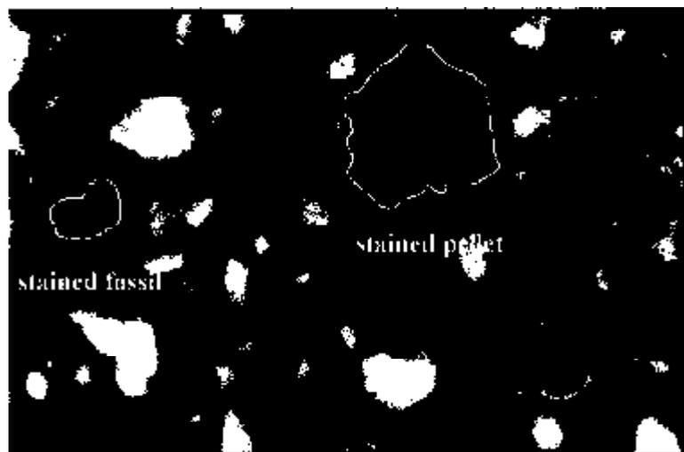
Plate 1. Photomicrograph (x100) of the thin section of the altered crust of cap rock as viewed under open nicol. The stained pellet and stained fossil are outlined. The major clastic constituents include quartz, plagioclase, fossils and pellets. The clastic components are inbedded in a matrix of clayey of unknown composition.
